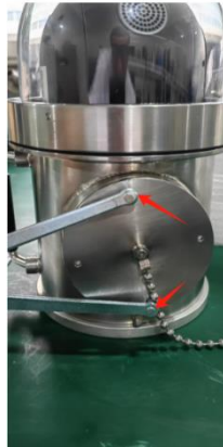
(1) Side cover hole position (2) Multi-purpose wrench into the side cover hole position (3) Multi-purpose wrench
