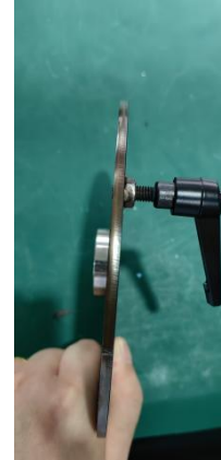
(3) jack wrench is installed on the suction cup
