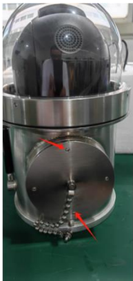
(1) Side cover hole position (2) Multi-purpose wrench into the side cover hole position (3) Multi-purpose wrench
